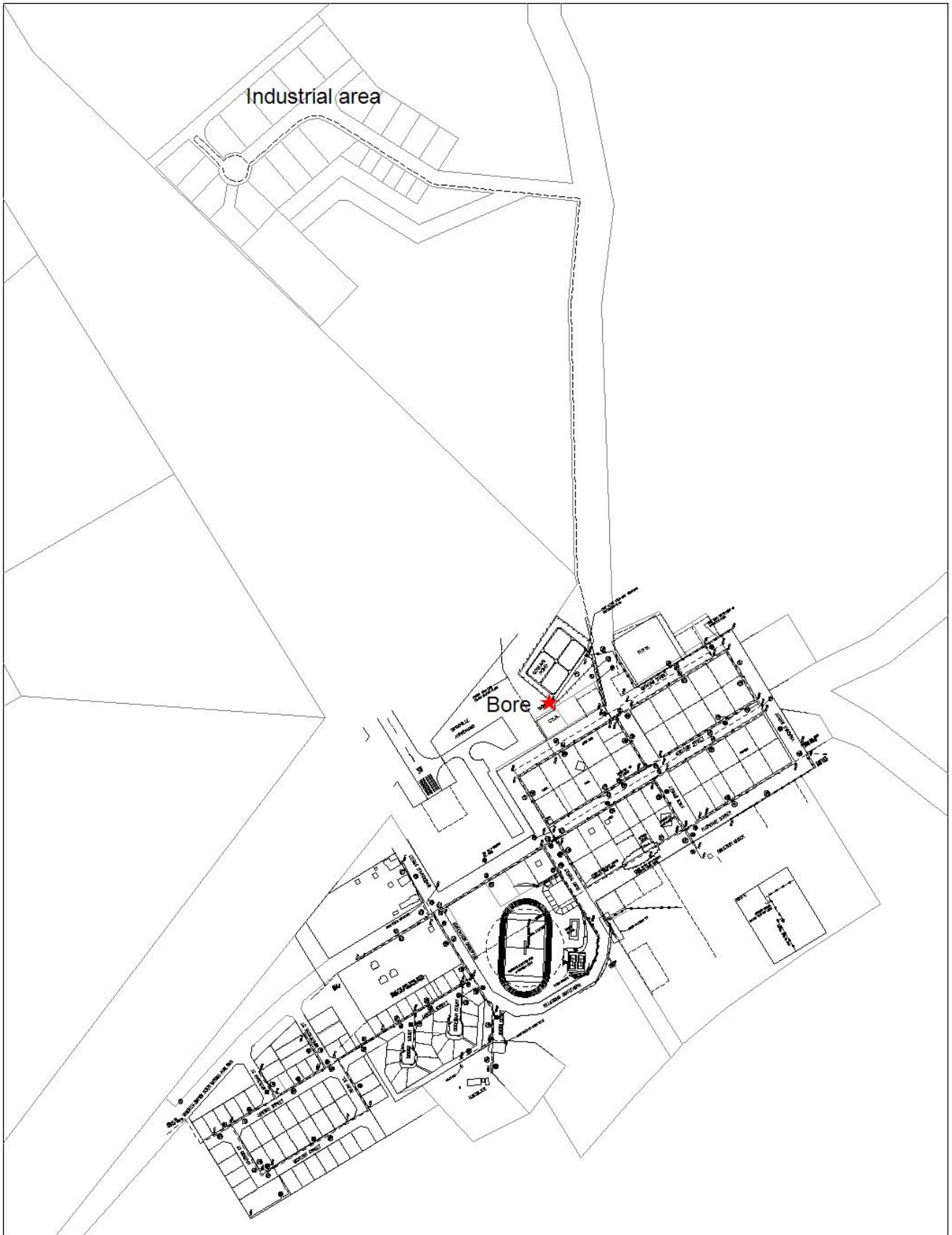
Figure 11: Birdsville drinking water supply schematics.
