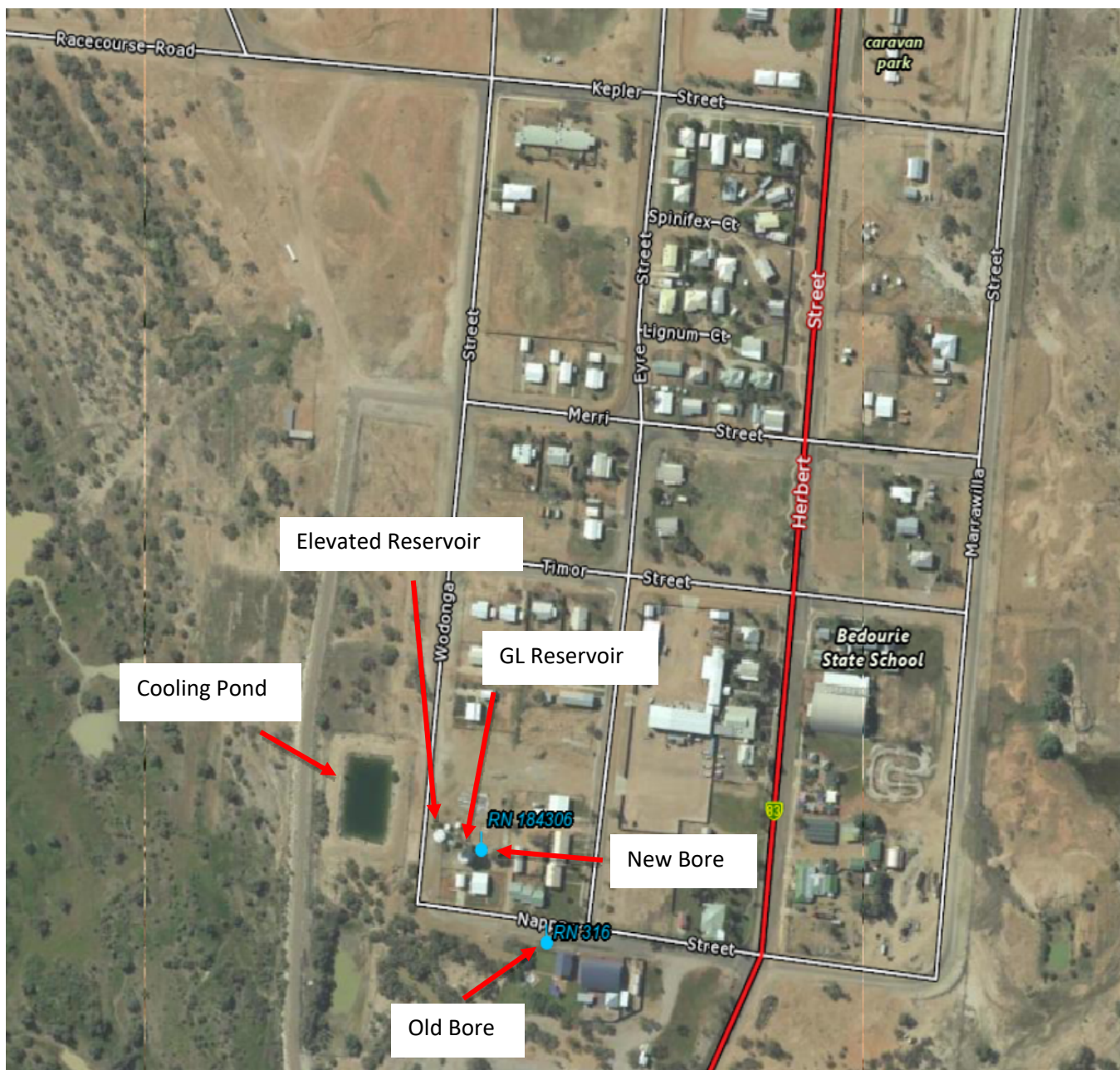
Figure 3: Annotated QLD Globe Image of Bedourie's Drinking Water Infrastructure.
