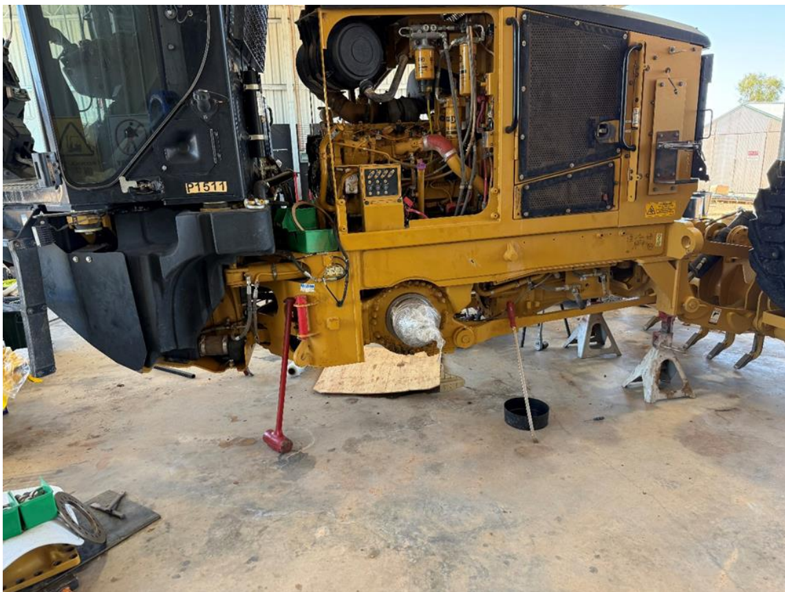
Tandem reseal on a 150 grader along with front main seal, cam box reseal, oil cooler reseal, new yoke an pinion seal
